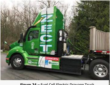
**Figure 24** – Fuel Cell Electric Drayage Truck (Photo curtesy of Ballard Power Systems)
