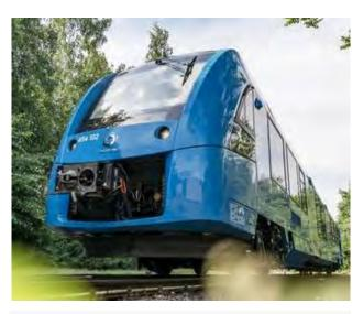
Figure 26 – Alstom Hydrail with Hydrogenics Engine (Photo courtesy of Alstom)<sup>2</sup>
